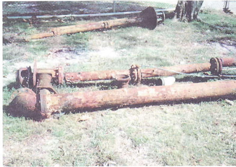
Photo 7 Corroded vertical shaft sewage pumps
