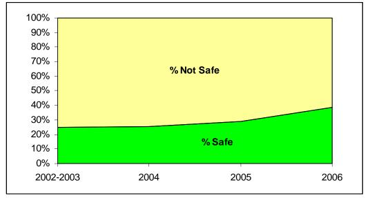
Figure 2.2 Results of EPA Outer Islands Water Catchment Bacterial Tests: 2002 to 2006
